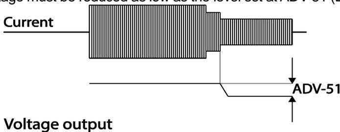
voltage before the energy saving operation starts will become the base value of the percentage. Manual energy saving operation will not be carried out during acceleration and deceleration.
