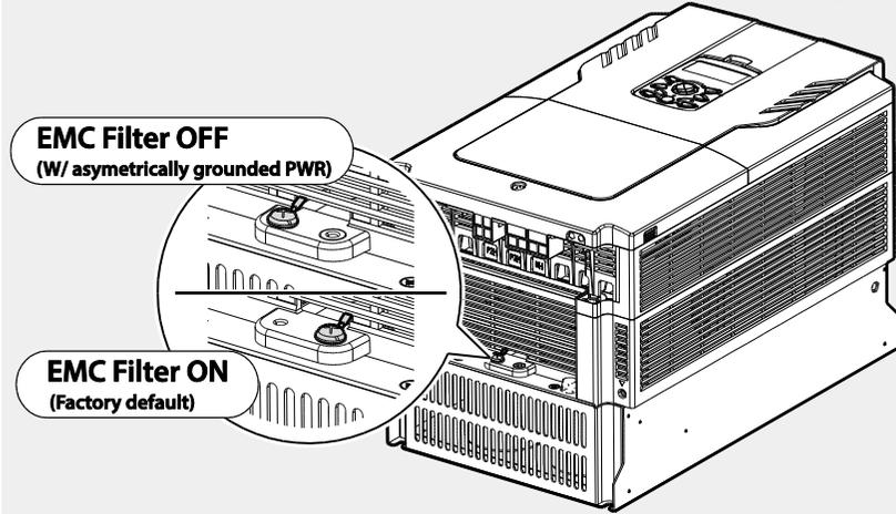
**Disabling the Built-in EMC Filter for 110–500 kW (3–Phase) Inverters**
