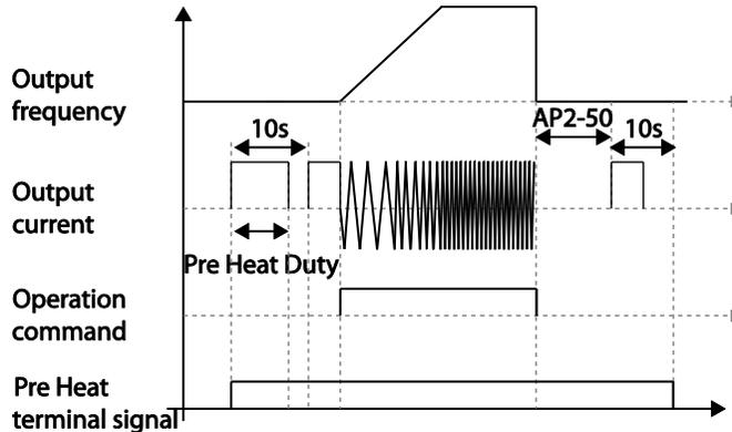
The diagram above shows the operation waveform related to AP2-50 DC Inj Delay T. The Pre Heat function performs when the inverter stop mode is set to Free Run and the Pre Heat signal is supplied. Then, if the inverter operation command is on, the inverter maintains acceleration and a fixed frequency. If the inverter operation command is off, the motor is in Free Run and the Pre Heat operations starts after the time amount set in AP2-50.
