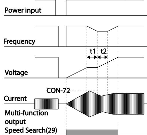
**Starting with power-on:** Set bit 4 to '1' and ADV-10 (Power-on Run) to '1 (Yes)'. If inverter input power is supplied while the inverter operation command is on, the speed search operation will accelerate the motor up to the frequency reference.
