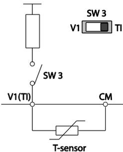
To receive PTC signal at V1 input terminal, set PRT-35 (Thermal InSrc) to '0 (Thermal In)' and set the Analog1 input selection switch (SW3) to T1.
