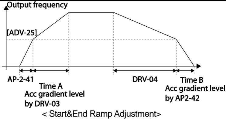
In the figure above, AP2-41 defines the acceleration time to the minimum operation frequency ADV-25 (Freq Limt Lo). AP2-42 defines the deceleration time from the minimum operation frequency to a stopped state. Time A (normal acceleration time set at DRV-03) and Time B (normal deceleration time set at DRV-04) in the figure will change according to the Acc/Dec gradients defined by AP2-41 and AP2-42.
