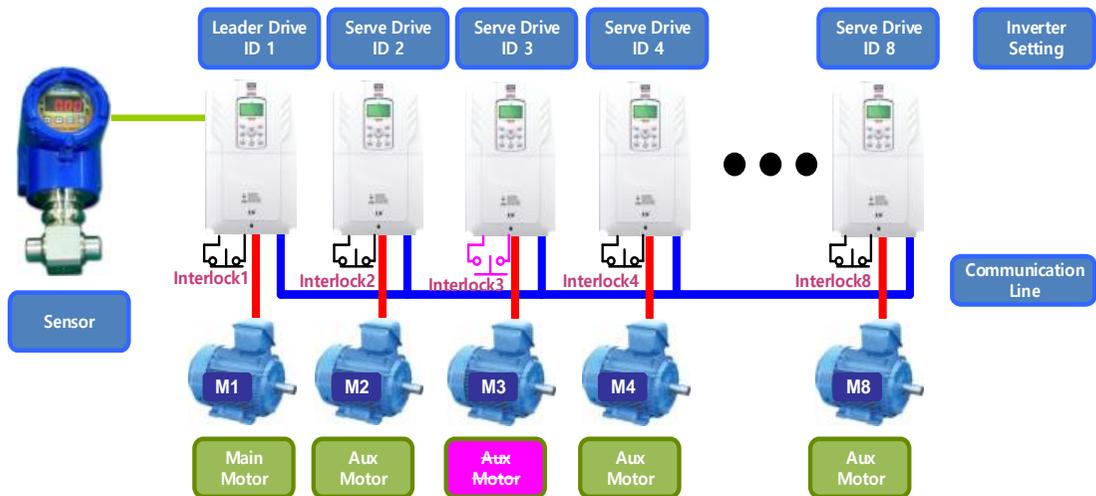
The picture below shows the function in case that M3 becomes HAND/OFF State or interlock and Trip are caused.(supposing that the priority is not changed),(interlock is the function corresponding to B terminal(Normal close)).
