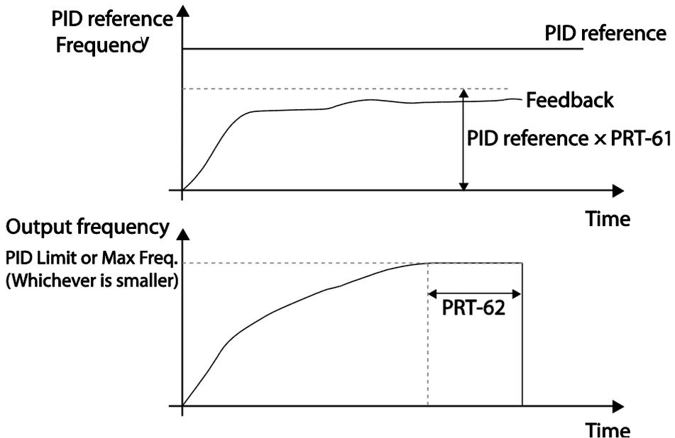
In the graph above, Pipe Break occurs if the feedback is smaller than the value calculated by multiplying the two values set at PID-04 and PRT-61(PID-04 x PRT-61) at the inverter's maximum output (when PID output is the maximum set value, or the inverter is running at the frequency set at DRV-20).
