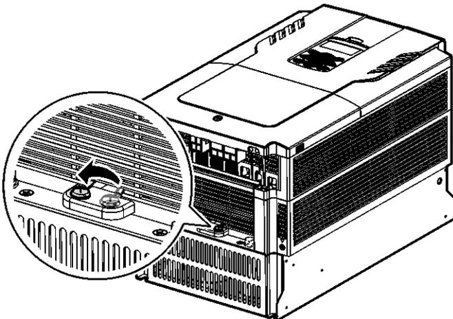
If the EMC filter is required in the future, reverse the steps and connect the EMC ground cable to the right terminal to enable the EMC filter.
