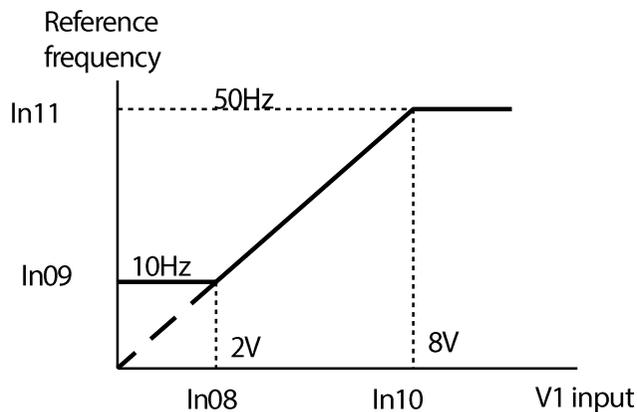
You can connect the terminal wiring as shown below. Refer to the In 07 –11 features.
