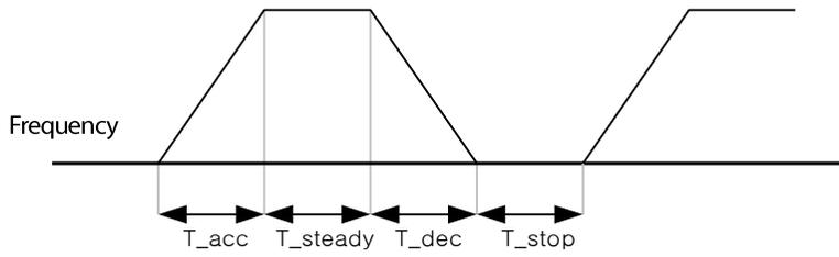
Example 2)  $Pr66 = \frac{T_{dec}}{T_{dec} + T_{steady1} + T_{acc} + T_{steady2}} \times 100[\%]$
