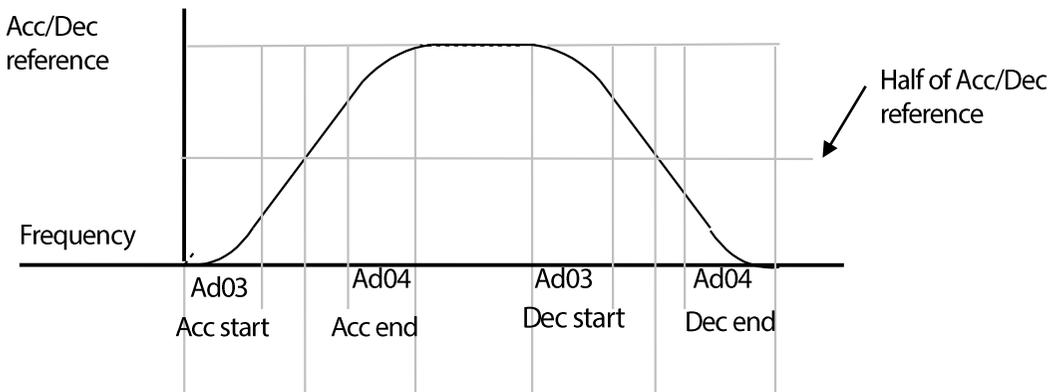
When Acc/Dec reference (bA09) is set to the maximum value while the goal frequency is lower than the maximum frequency, the S-curve is not created properly.
