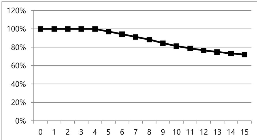
The 0.1 kW–0.2 kW products can be operated at a maximum of 50°C. However, the lifespan of the product may be reduced when operating continuously with a full load when the ambient temperature exceeds 40°C (35°C when an optional vent cover is installed).
