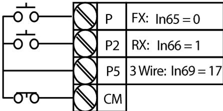
The 3-wire operation latches the signal input (the signal stays on after the button is released) as shown in the diagram above, and is used when operating the inverter with a push button
