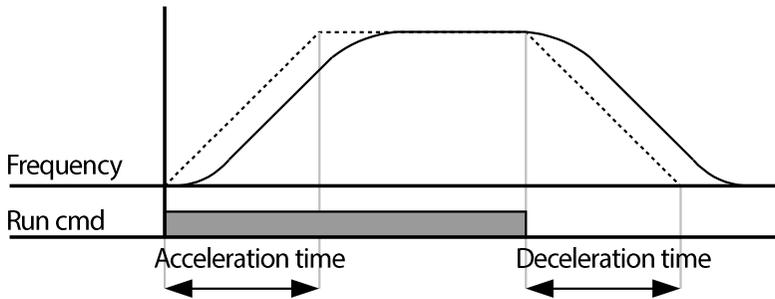
Ad03 defines the S-curve gradient level as a percentage, up to half of the total acceleration and deceleration (Acc Start and Dec Start) values. You can set the Ad03 parameter to a higher value to increase the gradient level for smoother acceleration and deceleration.
