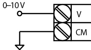
When the 0-10 V voltage is loaded from an external source
