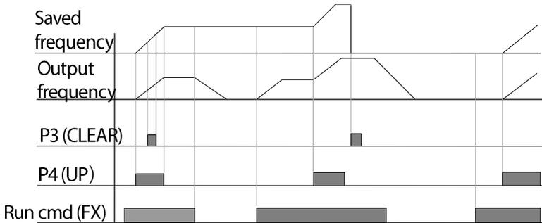
When the Ad66 code is set to 1: The motor accelerates by as much as the step frequency set by the Ad67 code at the multi-function input's positive edge that has been set as the Up terminal signal. The motor decelerates by as much as the step frequency set at the Ad67 code at the multi-function input's positive edge that has been set as the Down signal. The frequency is saved at the falling edge when the Up/down signal is specified. In this case,
