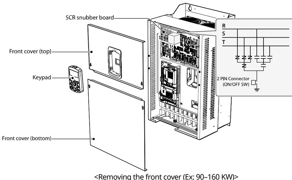
Refer to the following figures to locate the jumper switch on the SCR snubber board and install or remove the jumper cap to activate or deactivate the built-in surge filter.
