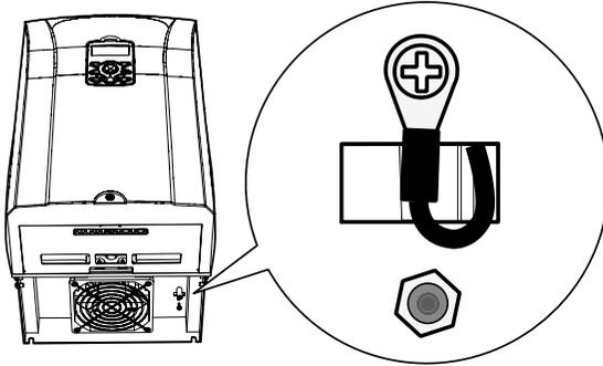
The EMC filter is deactivated if the EMC filter cable is connected to the insulated stud.
