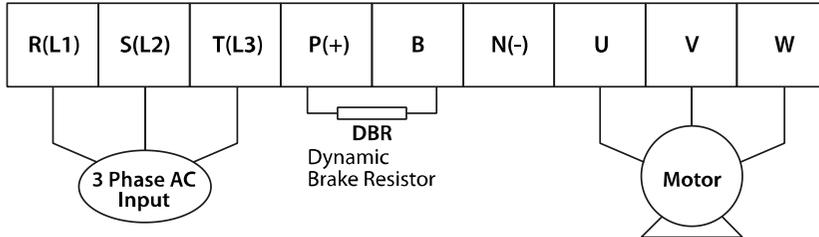
Connect the cables from the dynamic braking unit to the P (+) and B terminals to utilize the built-in dynamic braking unit.
