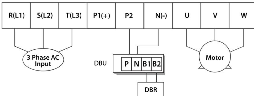
In 30-75 kW 200 V model types, the P1 and P2 terminals are connected with a jumper pin.
