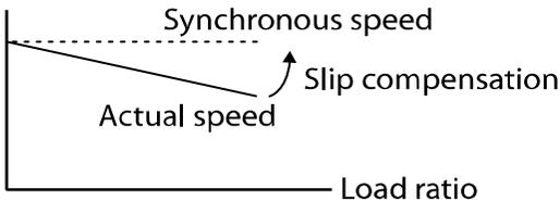
\*If DRV-09 is set to Sensorless, Vector, or V/F PG, the variation (slip) is automatically compensated.
