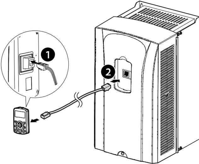
If a "Line Check" message is displayed on the keypad display and the keypad is not operating correctly after installing the remote cable, check the cable connection on both sides.
