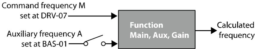
The auxiliary command frequency is turned off when the terminal input (Px) set to “40 (dis Aux Ref)” is on.
